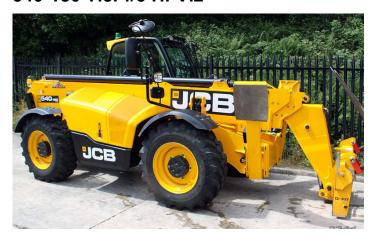
Max lift capacity 4,000kg Max lift height 17,510mm Max forward reach 13,340mm Capacity at maximum reach 550kg Engine power gross 75hp(55kW)
